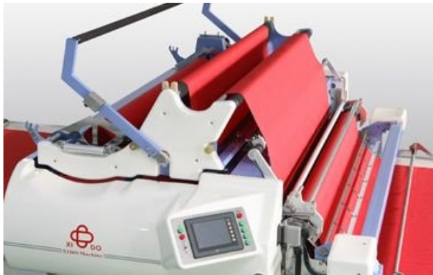
Tension-free spreading line
